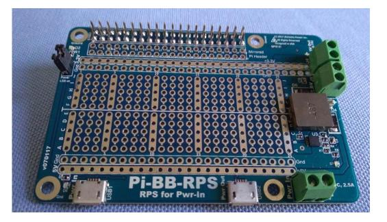
Pi-BB-RPS provides **<u>Redundant Power Supply</u>** capability. Second power is the micro-USB power. Power is switched seamlessly between these two sources. Priority is given to power source with higher power Voltage.
