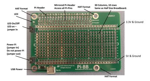
Pi-BB is a powered breadboard designed for the Raspberry Pi. Pi-BB offers the following:
