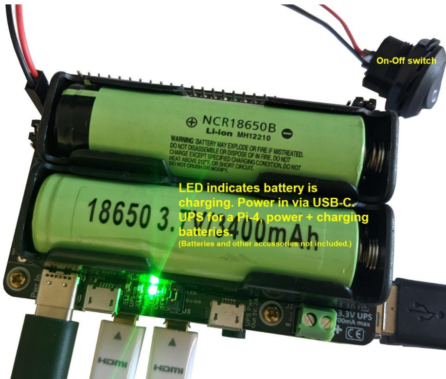
Pi-UpTime UPS 2.0 with On-Off Switch and charging LED on
