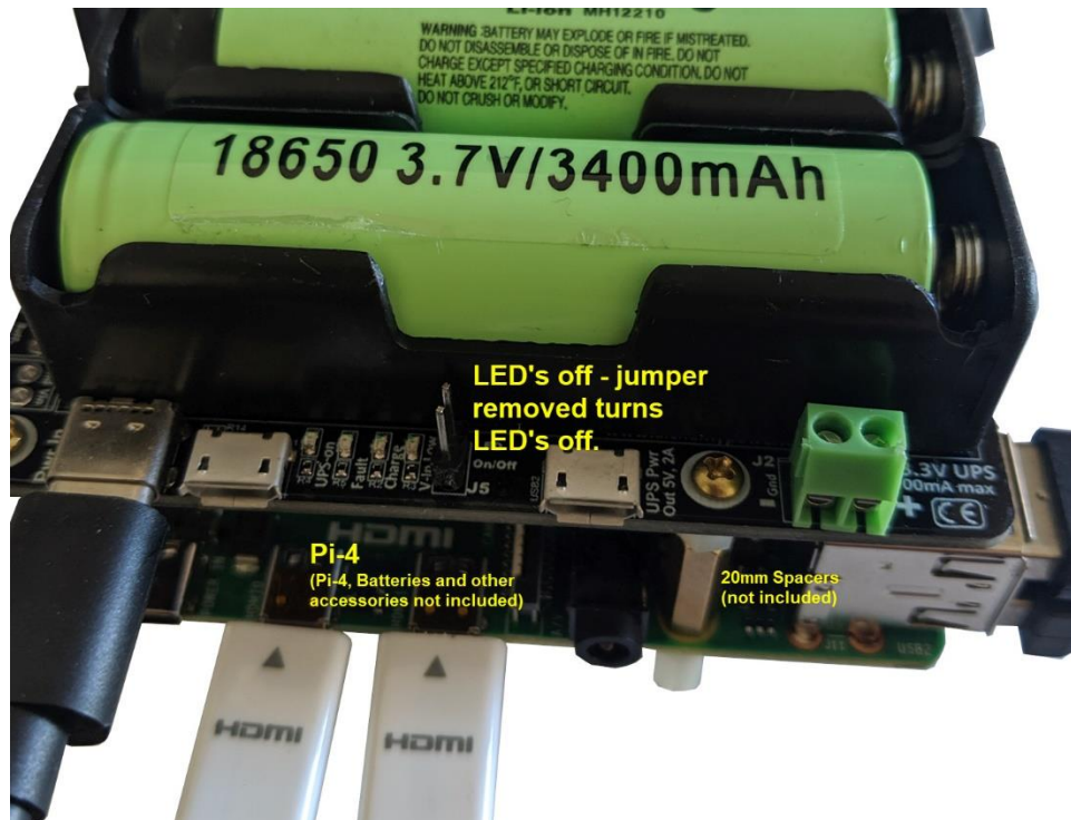
LED jumper is off, turning off all LED's. Shows mounted on a Pi-4 model
